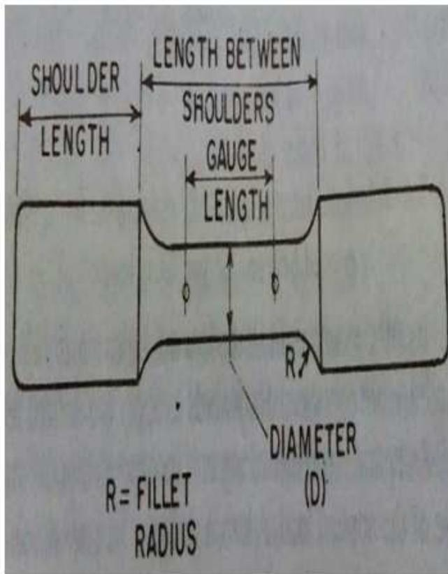
Figure 2: Tensile Test Specimen
